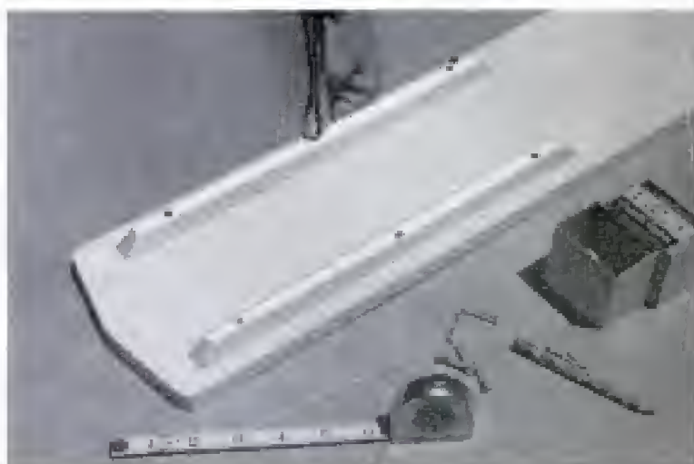
Each rudder is fastened 1 in. from back of ski and \frac{1}{2} in. from edge. Three 1-in. No. 6 screws are used
